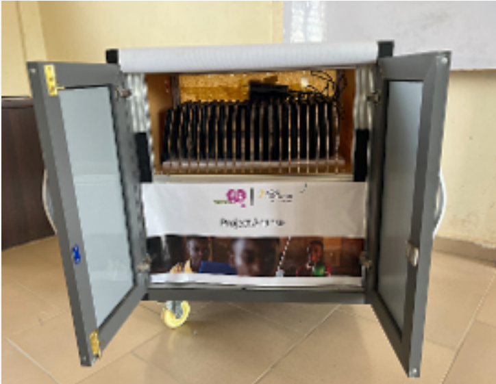
Since 2019, there are these mobile computer labs: small carts that can transport and charge 50 tablets.
